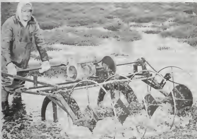
Figure 13: Harvesting fruit mechanically. (Left) Cranberry harvester used on a bog to loosen and float berries. (Right) Grape harvester straddling a row of Vitis vinifera or V. labrusca . The grapes fall on belts and are carried on escalators to the top of the harvester where they enter the arm to be deposited (at right) in a tractor-pulled bulk bin for processing.
